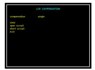
Selecting single compensation will conduct a zero compensation, short or open circuit at the same desired frequency that the test will be carried out at
