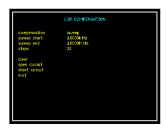
Sweep compensation needs to be configured exactly the same as the sweep details for the DUT to be tested. Frequency start, frequency end and steps all need to be replicated
