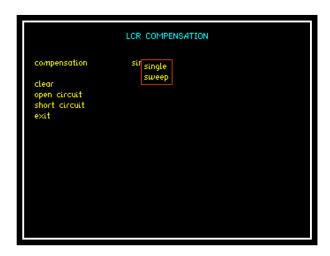
Select compensation parameter to correspond with test to be undertaken on DUT
