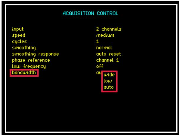
The bandwidth of the instrument usually set to "auto" can be forced to "wide" or "low". When not in auto selection, heterodyning is disabled and the bandwidth is either 5MHz wide or 100 KHz low to minimise noise when making measurements at low frequencies.
