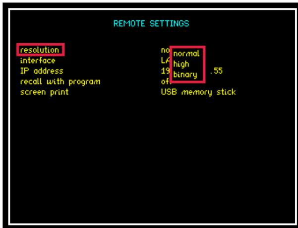
The default resolution setting for the PSM3750 is "Normal" this will set the Data Resolution to 5 decimal points plus any exponent eg: +1.2345+E00.
