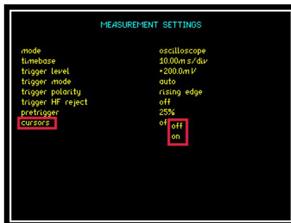
When enabled use the ▲ ▼ keys to enable and switch between Cursor 1 and Cursor 2.
