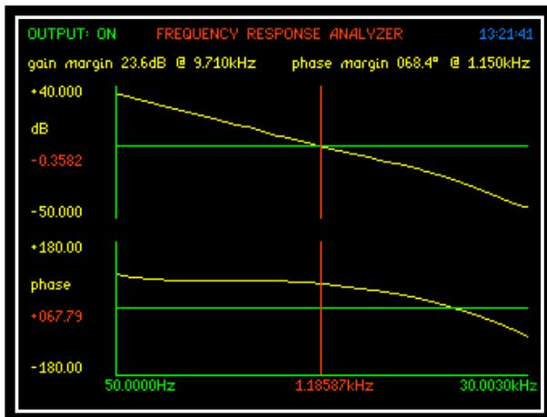
Moving from "TABLE" to "GRAPH" presents the same data but as a bode plot presentation, it can be noticed that a cursor is also present on the graph at the same frequency point as we saw in the table display above, using the  $\blacktriangleleft$   $\blacktriangleright$  arrows will move the cursor through the frequency sweep. Graph axes shown with max and min values of each axes plus the corresponding cursor value.
