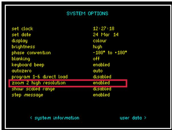
To set ZOOM 2 or 3 to high resolution, access the SYSTEM OPTIONS menu and scroll down to "zoom 2 high resolution" as shown. Press the ◀ key to enable this function.
