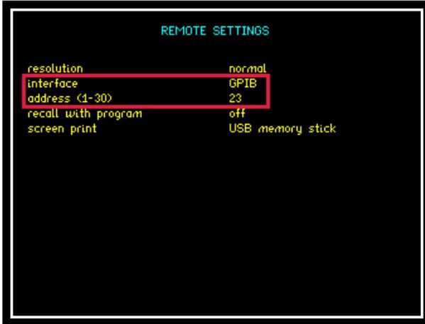
Configuring the instruments interface to GPIB will automatically set the IEEE address to 23 this can be changed within the address parameter in the range 0 to 30 (31 total possible addresses available).
