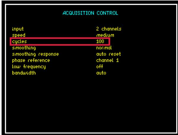
To change the number of complete cycles to be measured in each window between 1 and 100 either use the ◀ ▶ arrows or manually input using the numerical keypad and pressing "ENTER".
