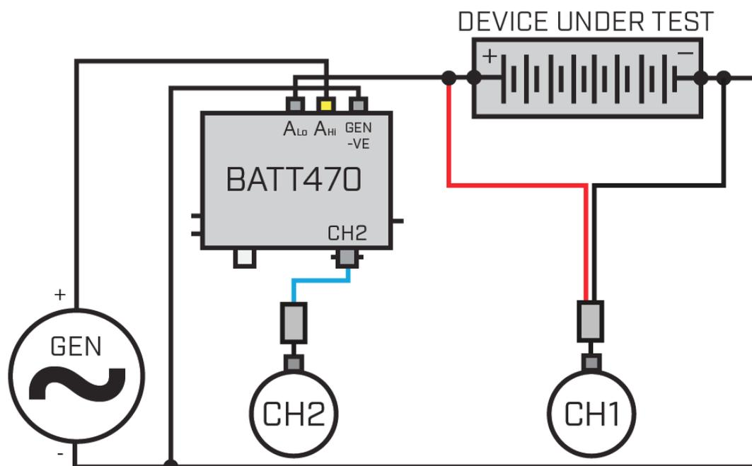
An impedance sweep can then be performed between the frequency limits of interest. This can be displayed in Nyquist form within PSMComm (EIS Mode) if preferred.
