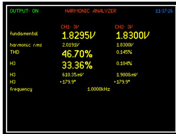
For the purpose of this manual the output signal was generated using the PSM3750's own generator as shown within the next screenshot, where it can be seen that the output frequency was set to 1 kHz.
