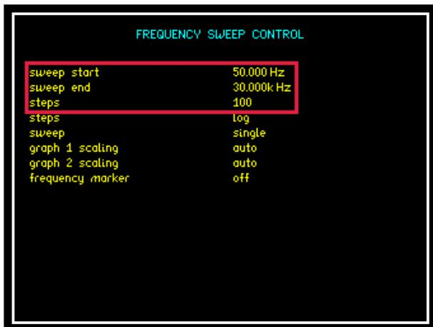
Enter "SWEEP" control mode by pressing the Sweep button. Set the start and finish frequencies that you wish to conduct your sweep across these can be inputted using the numerical buttons on the PSM's front panel. Set the amount of steps (Data Points) within your sweep to be displayed within the results screens.
