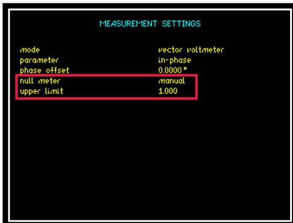
Selecting "manual" will allow the user to set their own upper limit to be displayed on the bar graph within the real time display as shown below.
