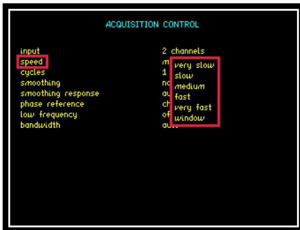
There are 5 pre-set speed options that adjust the nominal size of the window, and therefore the update rate and the time constant of the filter. Greater stability is obtained at the slower speed at the expense of a slower update rate.
