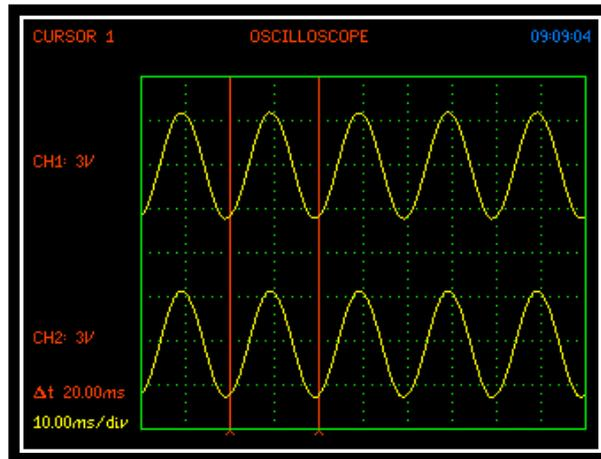
From the screenshot above (output set to 50Hz / 2Vpk) the display shows all fundamental measurements from the position of cursor 1. Also displayed is the time difference between the 2 cursors, "delta t" = 20.00ms with the timebase set to 10ms/div.
