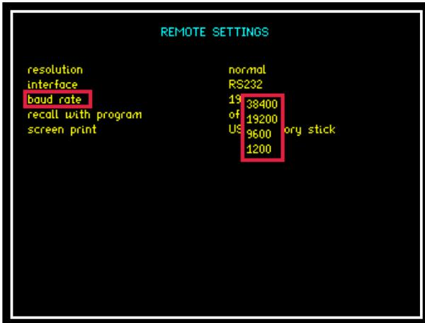
Selecting RS232 will then open up the "Baud Rate" option. Select an applicable data speed rate from the 4 options given in the drop down menu (Default Setting is 19200).
