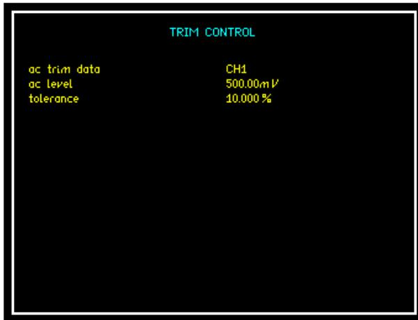
Selecting the ac trim data to be CH1 we can set the ac level at 500mV with a tolerance of 10%
