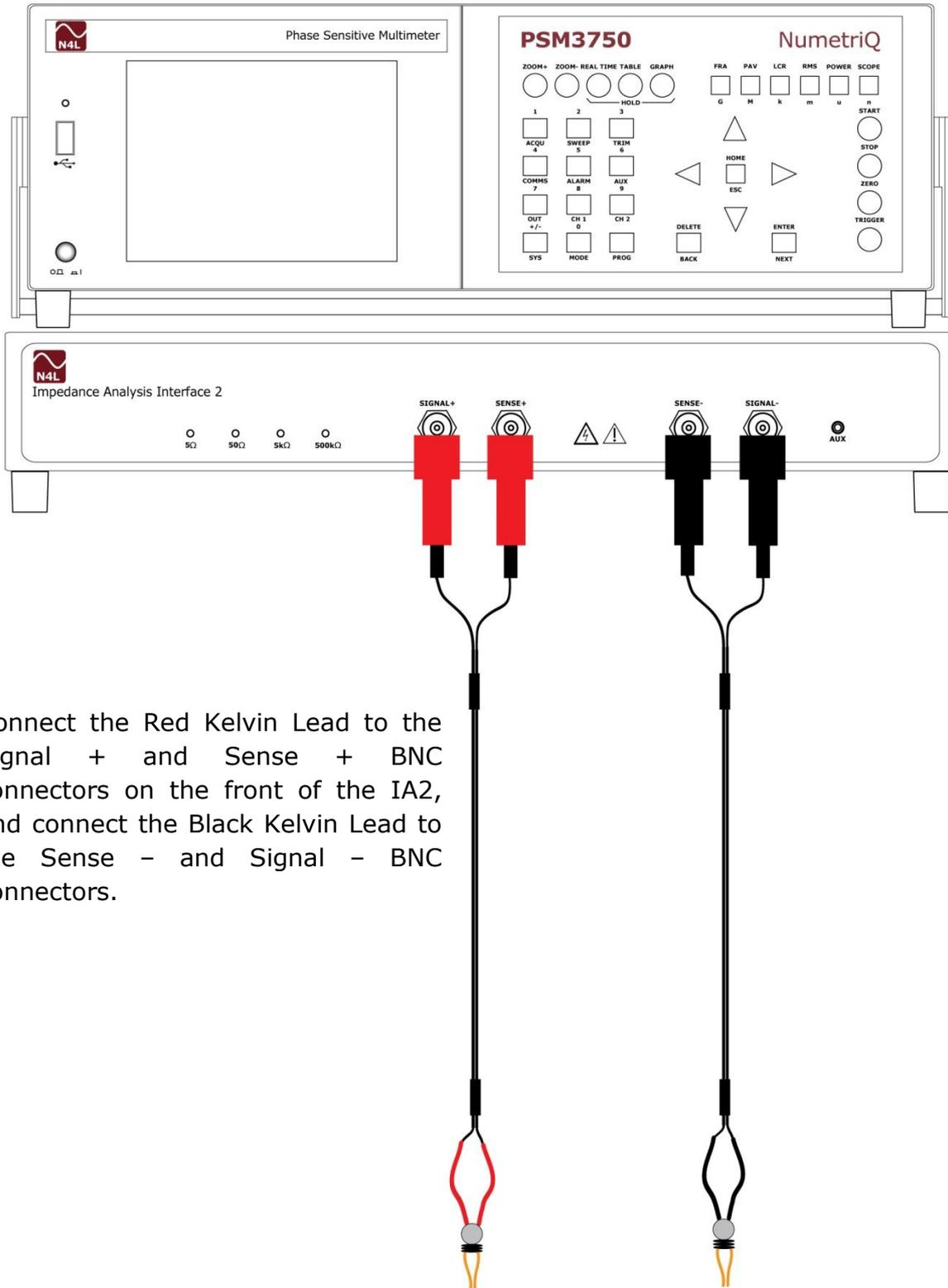
Connect the Red Kelvin Lead to the Signal + and Sense + BNC connectors on the front of the IA2, and connect the Black Kelvin Lead to the Sense - and Signal - BNC connectors.
