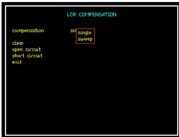
Select the compensation parameter to correspond with the test to be undertaken on the DUT.
