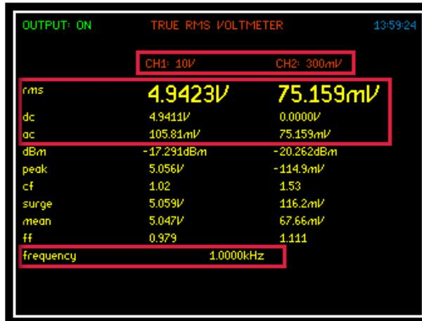
From the RMS Voltmeter display screen we can see the 2 sets of measurements from the same input. CH1 is displaying both the ac+dc components of the input signal with the ranging set onto the 10V scale.
