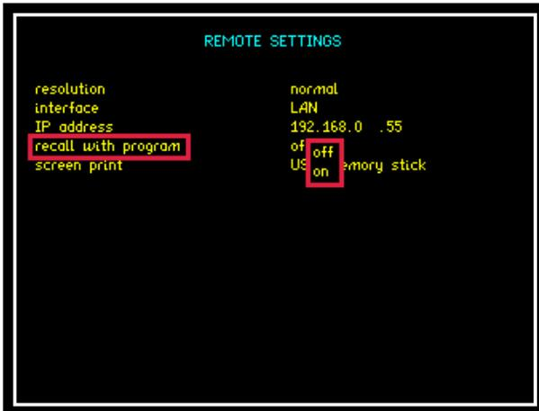
The recall with program parameter will allow any pre-set Comms configuration to be recalled if saved along with a nominated program within the "PROG" settings. To recall a Comms configuration set the recall option to "ON" then recall the appropriate program (Remember to set this first before recalling your saved program).
