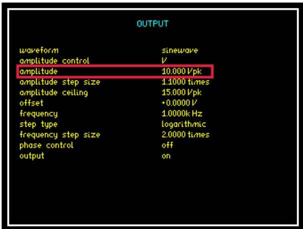
The "OUT" mode refers to the PSM3750 output generator. Information relating to all of the outputs parameters can be found in section 4.1
