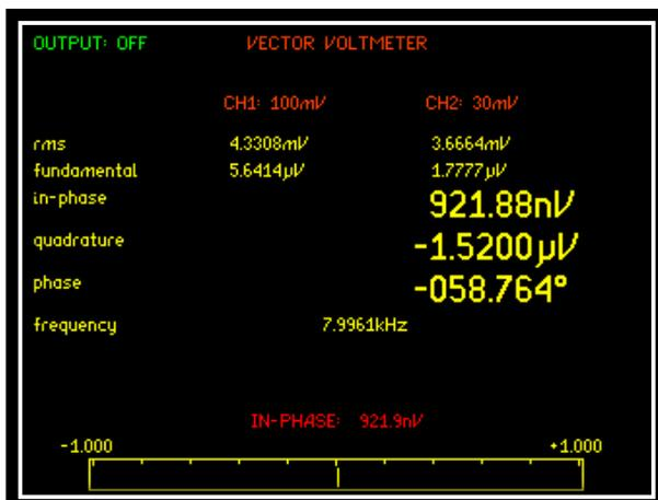
Within the "Real Time" display we now have the null meter at the bottom of the screen with limits shown as 1 as set within the previous screenshot.
