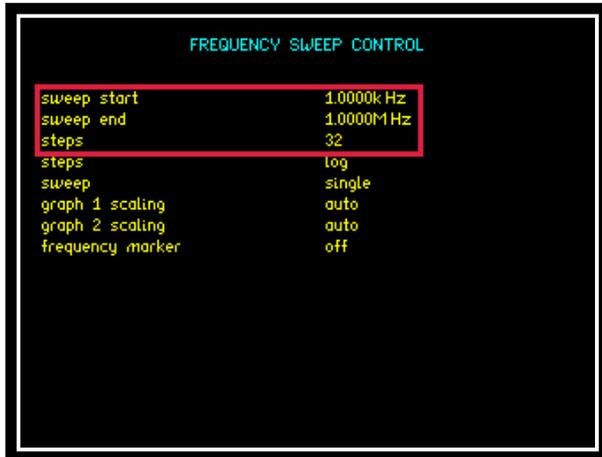
Setting the “steps” parameter to log or linear will show how all the data points will be displayed within the resultant graph display.
