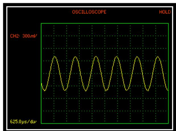
Viewing both channels within the Oscilloscope mode it is clear that by setting the coupling to ac only, the same ac waveform is much more visible within CH2's screenshot.
