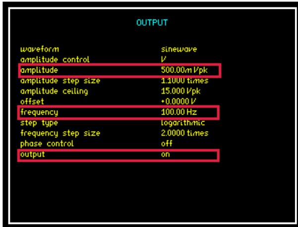
Within the "OUTPUT" mode set the amplitude parameter to the peak voltage signal required from the instruments generator. Frequency can be set to display the on screen measurements at this stated frequency, once all parameters are set then change the "output" to ON.
