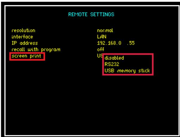
The Screen Print option will allow any screen display on the PSM3750 to be copied either to an RS232 printer or USB memory stick, select the appropriate transfer method required or alternatively this parameter can be disabled. To print the screen display press and hold the "START" button for 3 seconds. A BMP file will be transferred to the memory stick.
