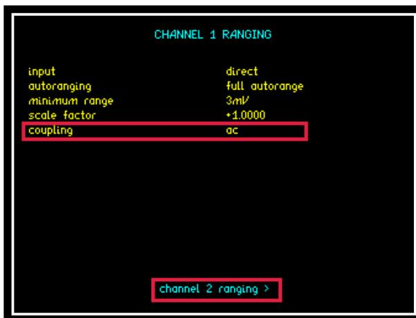
Within the CH1 /CH2 menu set the coupling to ac only as described in an earlier section called "FRA Sweep with ac Coupling". Pressing
