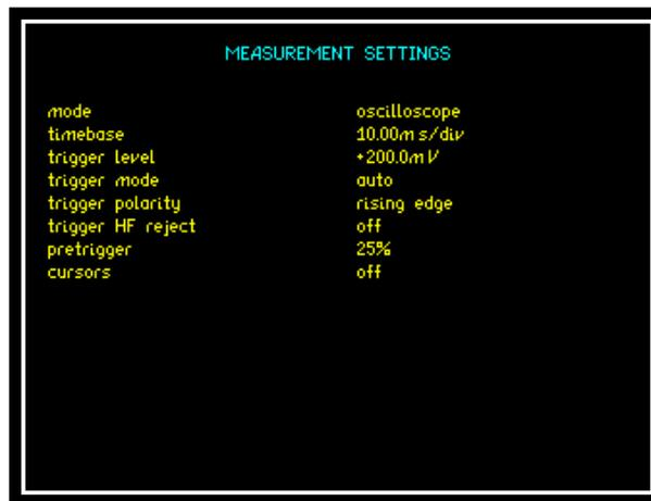
**Timebase:** The display for the oscilloscope is divided into 10 divisions along the time axis with the selected timebase displayed in the bottom left hand corner of the display. The timebase may be set to any real value between 15 $\mu$ s/div to 5s/div. Pressing the ◀ ▶ arrows on the main panel will adjust the timebase by a factor of 2.
