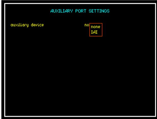
Press the "AUX" key on the PSM3750. The auxiliary device will appear as shown from the dropdown menu, select IAI and press "ENTER" to confirm.
