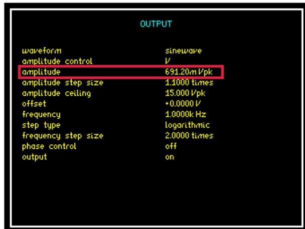
This will now be the maintained measured voltage or current and will allow a much more controlled level over changing levels such as a frequency sweep
