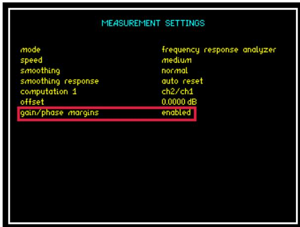
Enter "FRA" mode by pressing the FRA button. Use the ▼ arrow until the red box surrounds the gain/phase margins parameter now press ◀ arrow to enable this function, these parameters will now be displayed within the graph results display as shown later in this section.
