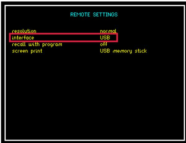
To use a USB lead to connect, set the interface parameter to read "USB".
