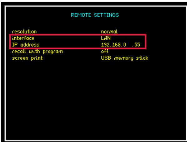
Configuring the interface to LAN will then display the IP address applicable to your instrument. This address will be required upon connection to any software to enable correct connection to the instrument; this is changed using the numerical keypad.
