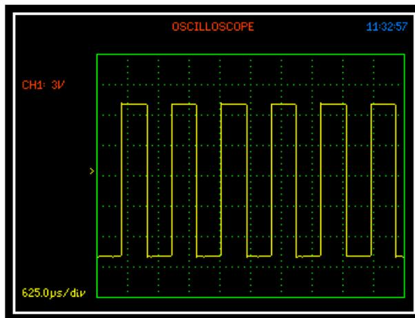
Here we are able to view the squarewave signal that was previously set within the "OUTPUT" menu screen and which was being analyzed for this guide.
