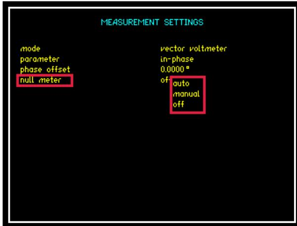
To activate the "null meter" function press the "PAV" button and then press the ▼ arrow until the red box surrounds the null meter parameter, press the ► arrow to open up the drop down menu as shown. Select either "auto" or "manual" range.
