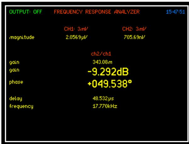
Due to the fact that the PSM3750 generator is switched off by default, the display may read some random values due to noise pick up as shown.
