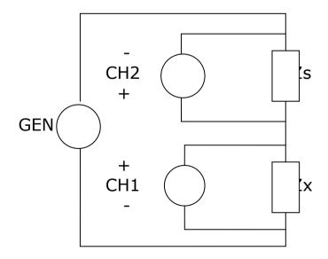
For "shunt" connection, shown above, the current is measured directly across the shunt using CH2 while the voltage across the Zx is measured by CH1. Notice that the positive inputs to both CH1 and CH2 are connected to the midpoint to minimise common mode loading effects.
