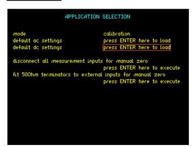
By selecting the 'default dc settings' option via the ▼ key followed by the ENTER key, the PPA will be configured correctly for DC calibration.
