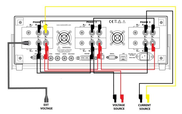
Where it is not possible to generate reference voltage and current signals at the same time, it is still recommended that voltage or current signals are applied to all 3 respective inputs.
