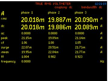
Here we have applied a nominal 20mAdc to all three direct current inputs. This is 60% of range 1 on a standard PPA5530.
