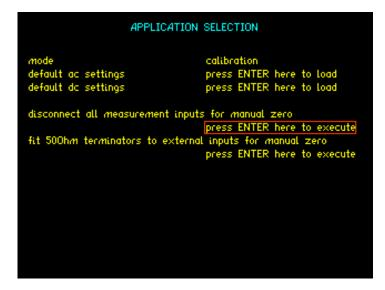
In most cases, calibration will be associated with direct voltage or current inputs, therefore the first manual zero option shown here will be the one most commonly used.
