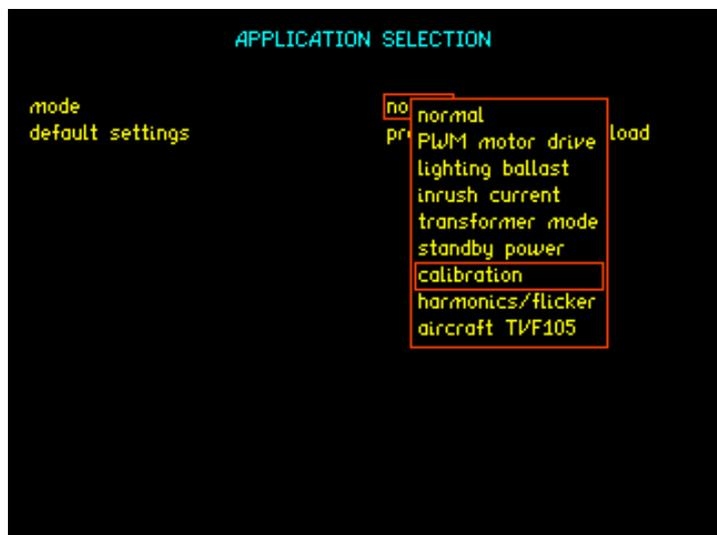
In order to simplify instrument configuration during calibration, the application menu (APP button on the PPA front panel) includes a calibration option as shown here.
