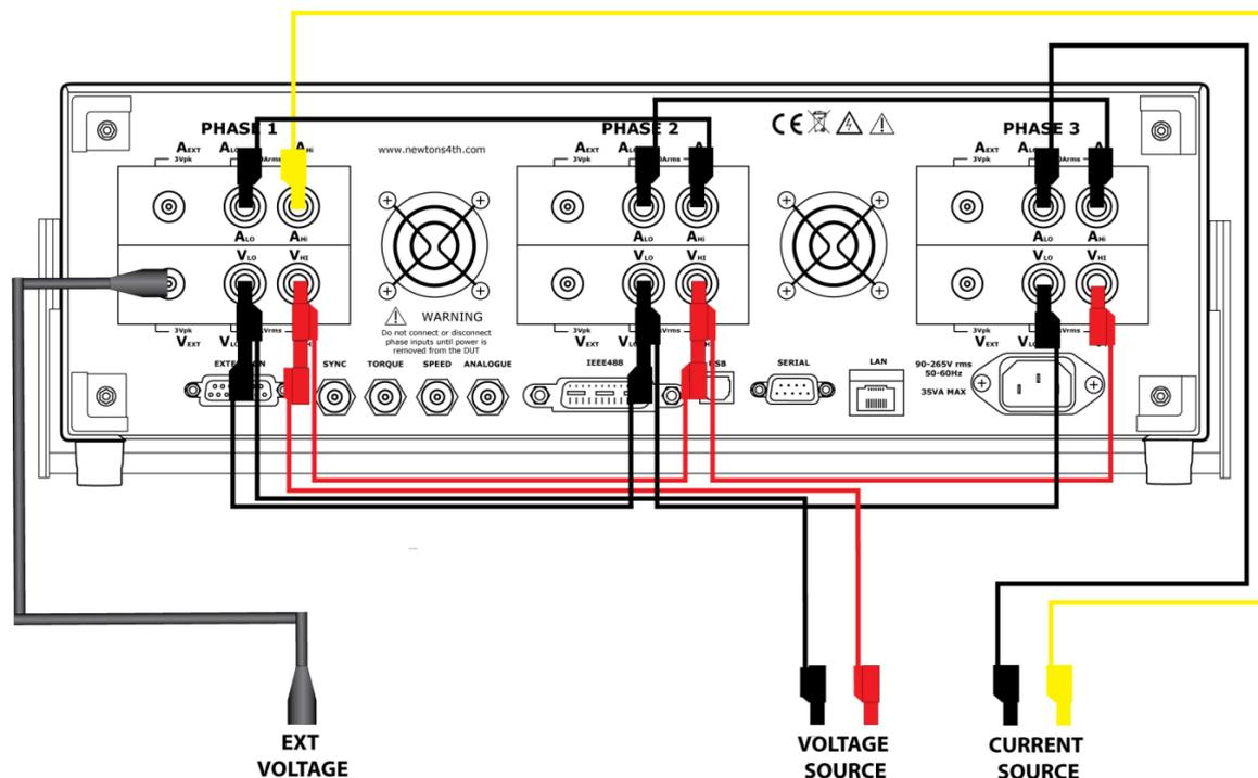
Where it is not possible to generate reference voltage and current signals at the same time, it is still recommended that voltage or current signals are applied to all 3 respective inputs.
