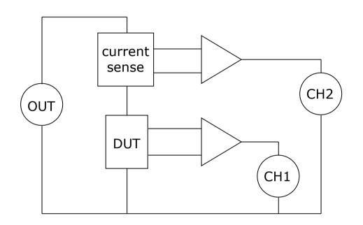
The IAI2 has 4 selectable 'shunts' to sense the current through the device under test:
