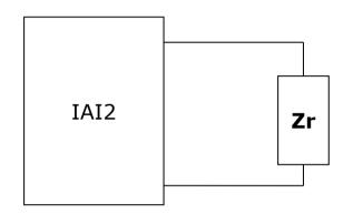
Then, if **ZI** is the impedance measured by the IAI2 with the known reference impedance **Zr** connected and **Zm** is the impedance measured by the IAI2 with the DUT connected:
