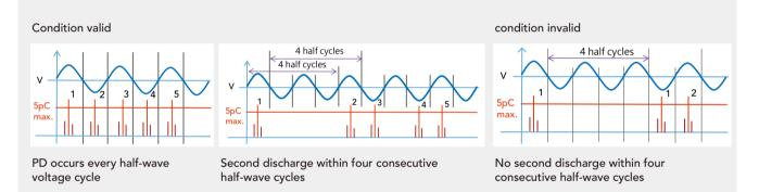
Example Description - The number of PD failures is set to 5 P.D
