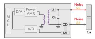
PD testers of other brands: Elongate the test cable to make contact with the DUT, which allows for interference due to the high frequency radiation in the surrounding environment, resulting in inaccurate measurements.
